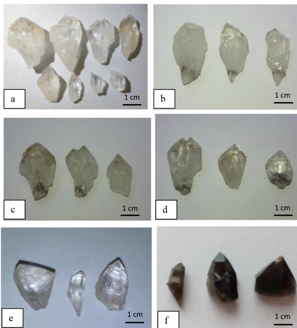
Fig. 1. a) Quartz crystals of the EQ region before irradiation. b) Crystals of the EQ produced by irradiation till 100 kGy. c) Crystals of the EQ produced by irradiation till 200 kGy. d) Crystals of the EQ produced by irradiation till 300 kGy. e) Quartz crystals of the SWA region before irradiation. f) The crystals belonging to the SWA that are completely colored with smoky color (They are irradiated from left to right at 100, 200 and 300 kGy).
